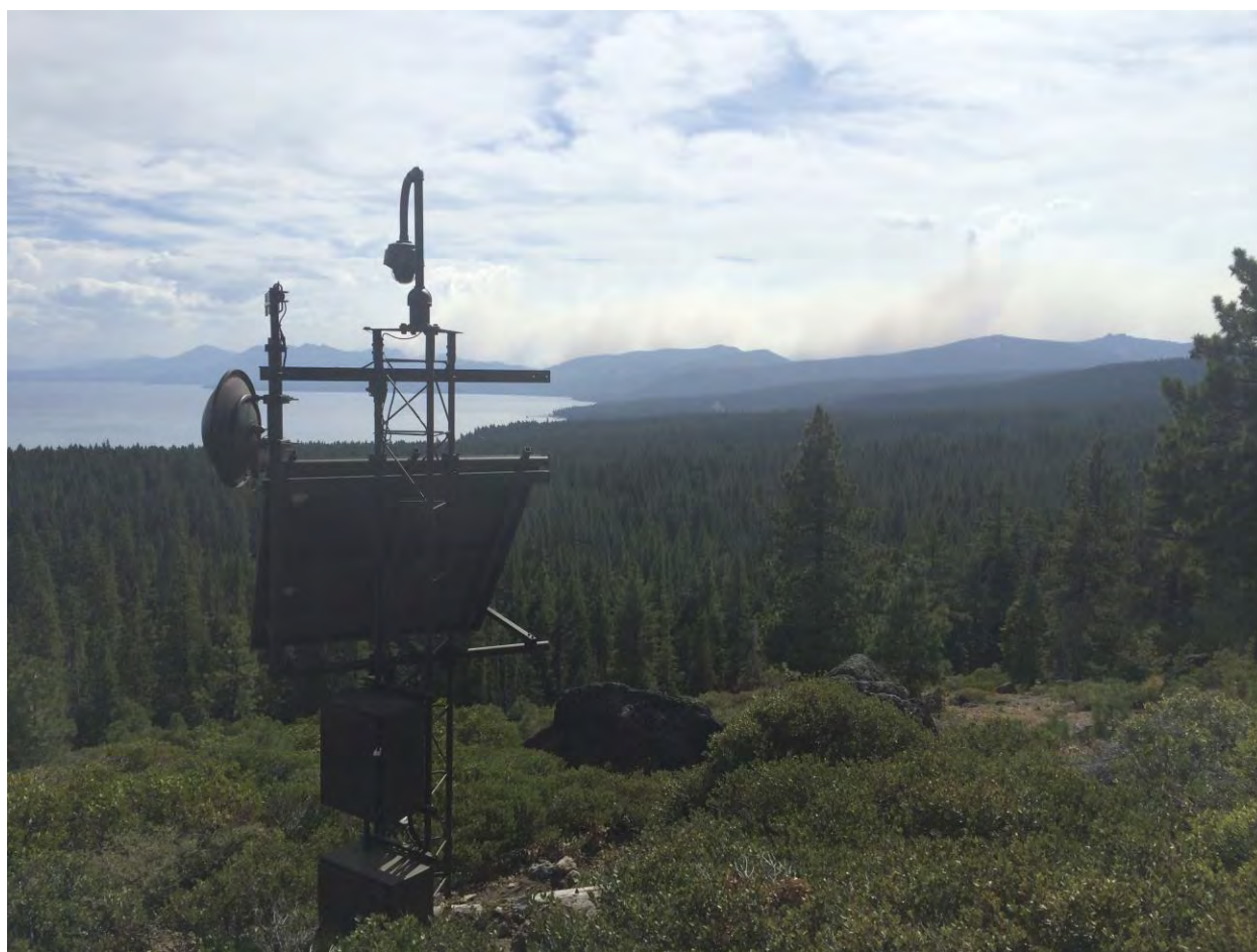
Figure 2. A combined earthquake early warning ShakeAlert and ALERTWildfire station in the Tahoe basin near Dollar Point, California
